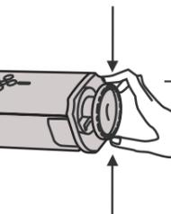
d) Put the inner sleeve back into the sleeve holder and make sure the plastic ring sits in the groove.
